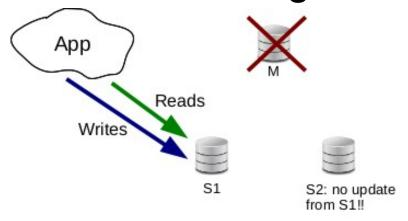
Need to set up replication between S1 and S2
